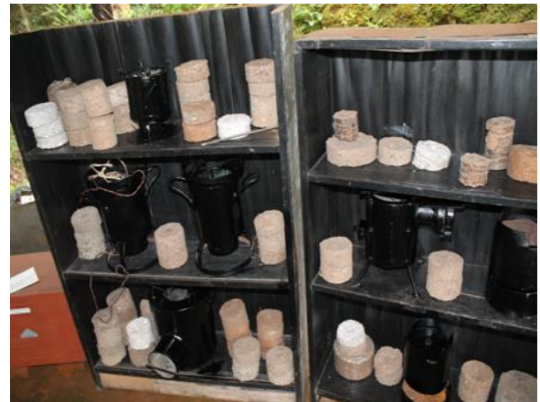
Photo 3: Briquette production from compressed charcoal, waste materials, saw dust, papers, etc.
